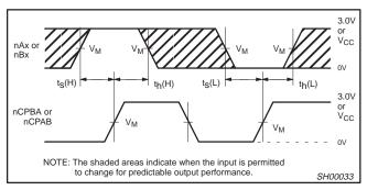
Waveform 4. Data Setup and Hold Times
