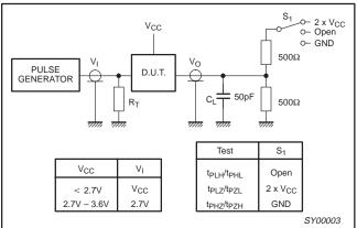
Load circuitry for switching times
