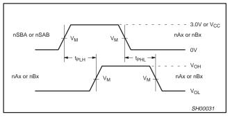
Waveform 2. Propagation Delay, nSAB to nBx or nSBA to nAx, nAx to nBx or nBx to nAx
